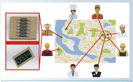
Sensors arrays implemented on textiles and interfaced with flexible electronics can report the location of positives and identify sources of the outbreak.
